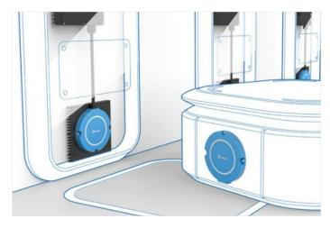
Autonomous AGVs can locate available charging stations and charge wirelessly, with no human intervention.
